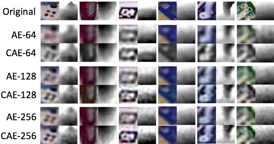
Fig. 7. RGB-D patch reconstruction comparison between our AE and CAE for a given feature dimensionality F . Clearly, the AE and CAE focus on different qualities and both networks increase the reconstruction fidelity with a wider compression layer.
